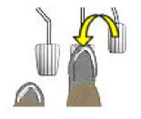
Quick, firm and progressive braking Clutch in at last moment
